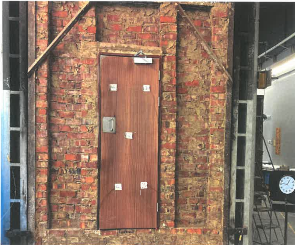
Photo 6: At 47 min, door still intact
