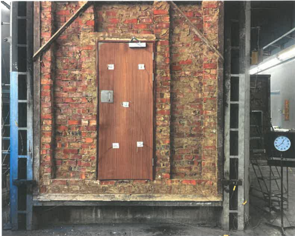
Photo 4: At 39 min, door still intact
