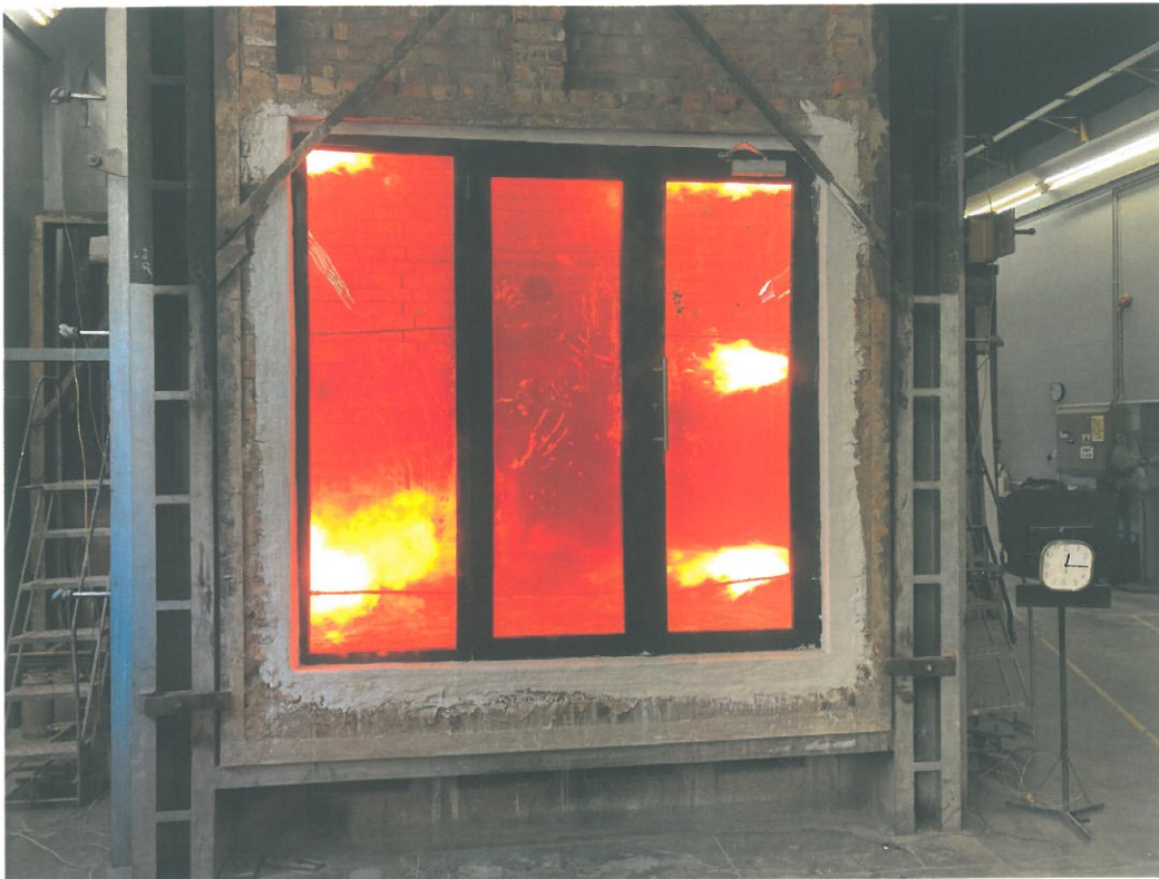
Photo 4: Photo taken of the unexposed side of the system at 30 minutes.
