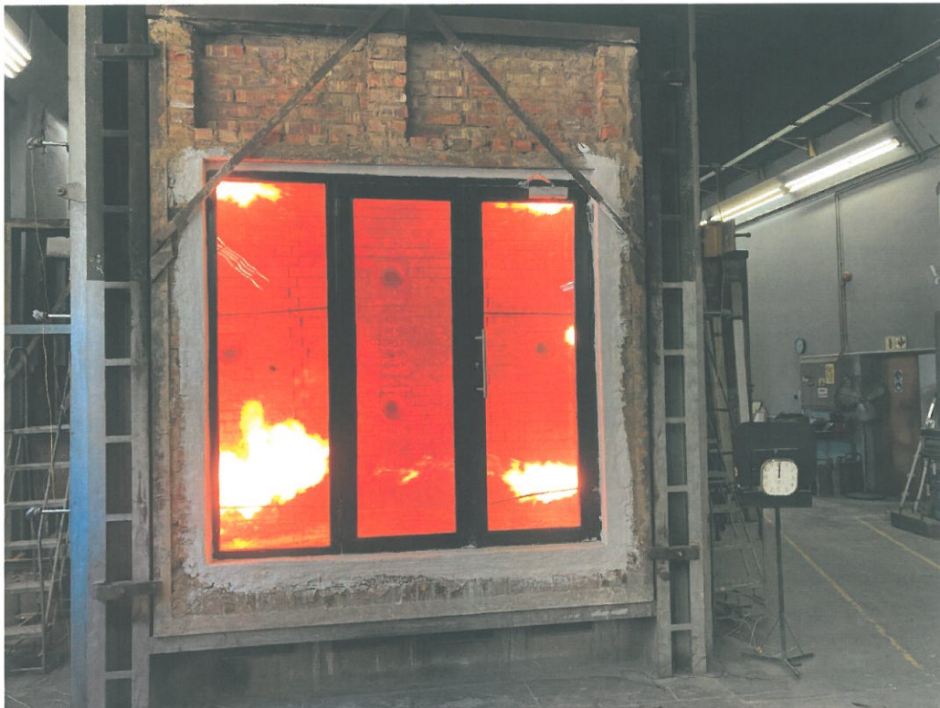
Photo 2: Photo taken of the unexposed side of the system when the test commenced.
