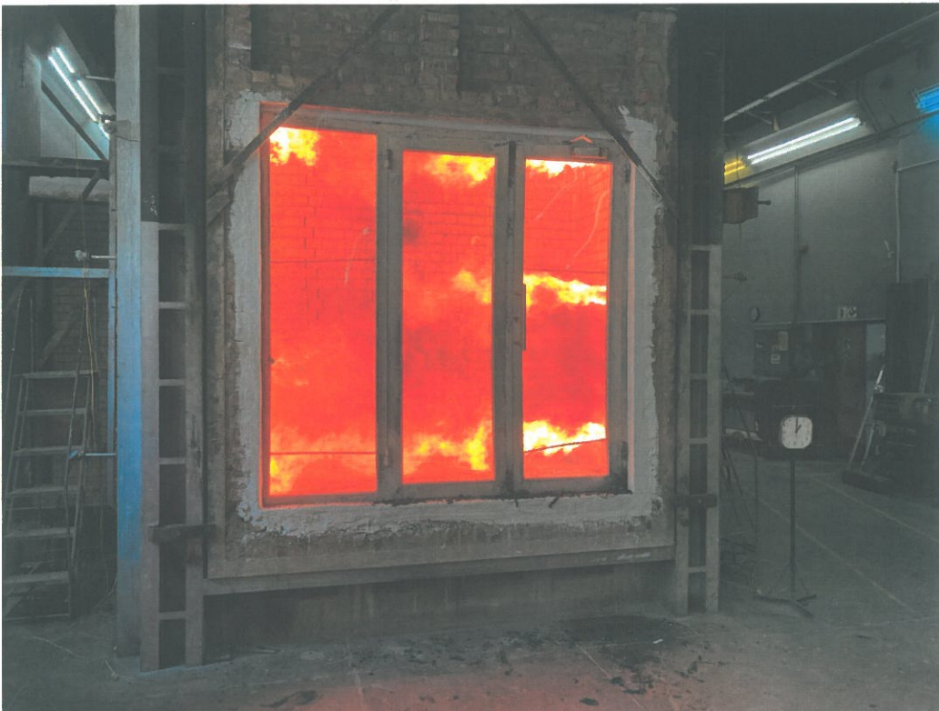
Photo 6: Photo taken of the unexposed side of the system at 60 minutes.
