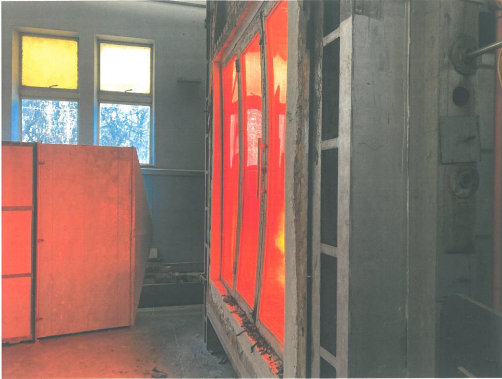
Photo 8: Photo taken of the unexposed side of the system at 80 minutes. Note smoke (unburnt diesel fumes) visible inside furnace due to anomaly at 71 minutes.
