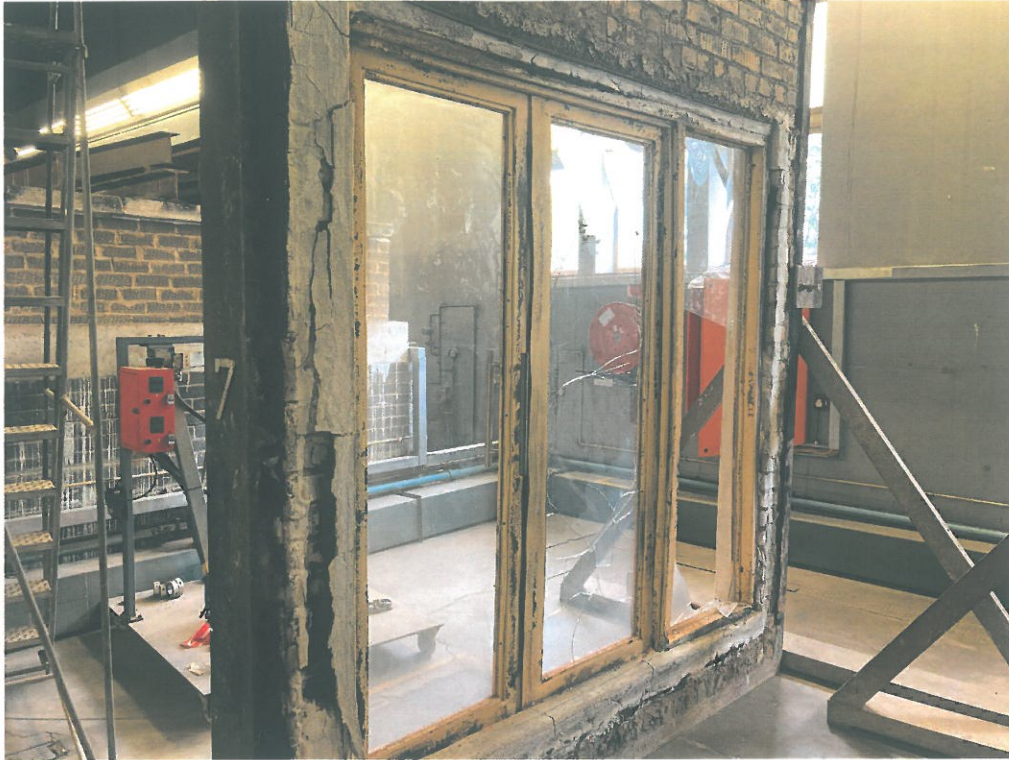
Photo 9: Photo taken of the exposed side of system after termination of test and removal from the furnace. The cracks and holes visible on the glazing only formed after test termination when the class cooled down.
