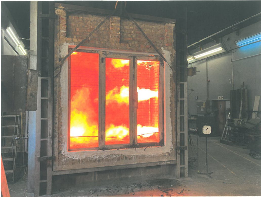
Photo 6: Photo taken of the unexposed side of the system at 60 minutes.
