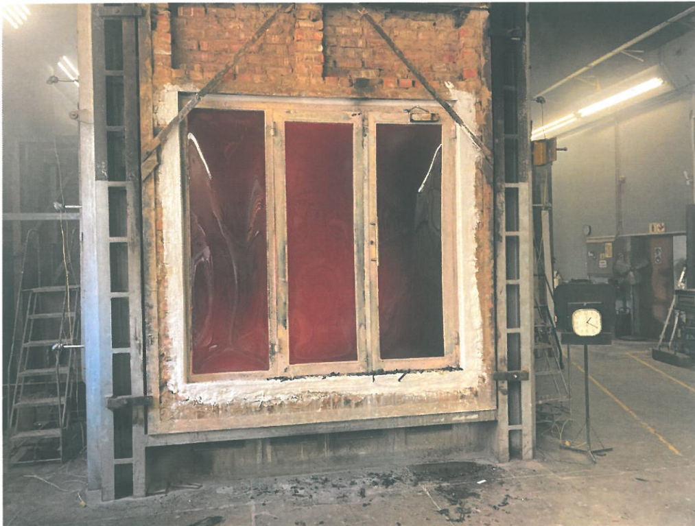
Photo 8: Photo taken of the unexposed side of the system at 80 minutes. Note smoke (unburnt diesel fumes) visible inside furnace due to anomaly at 71 minutes.
