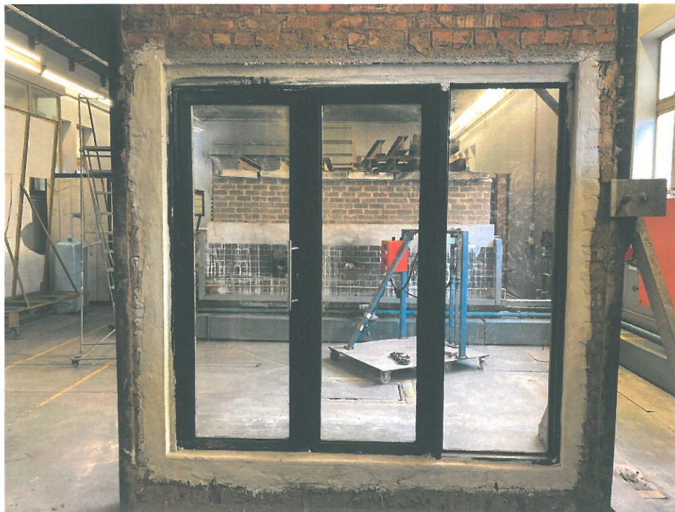
Photo 1: Photo of the exposed side of the specimen prior to testing.
