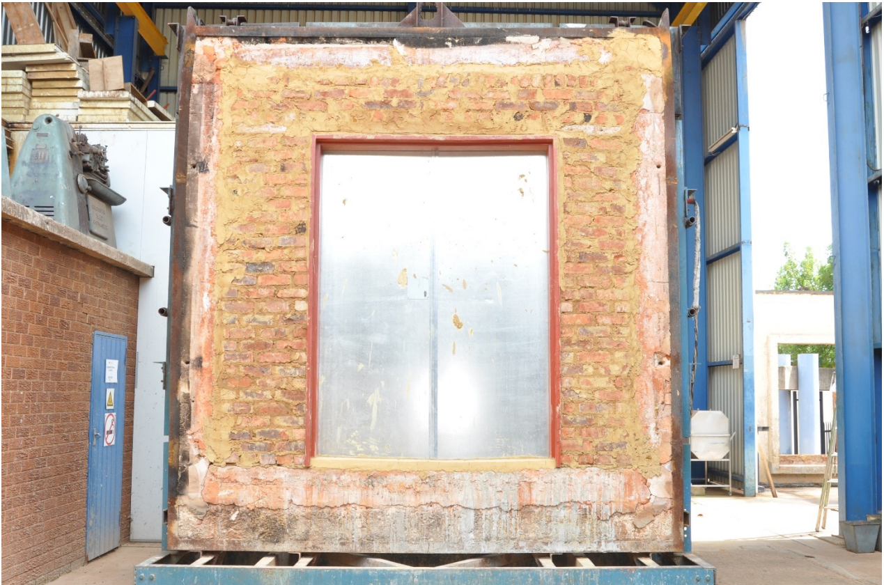
Figure 2.1: The Rocklite Class D Double from the exposed side prior to the test
