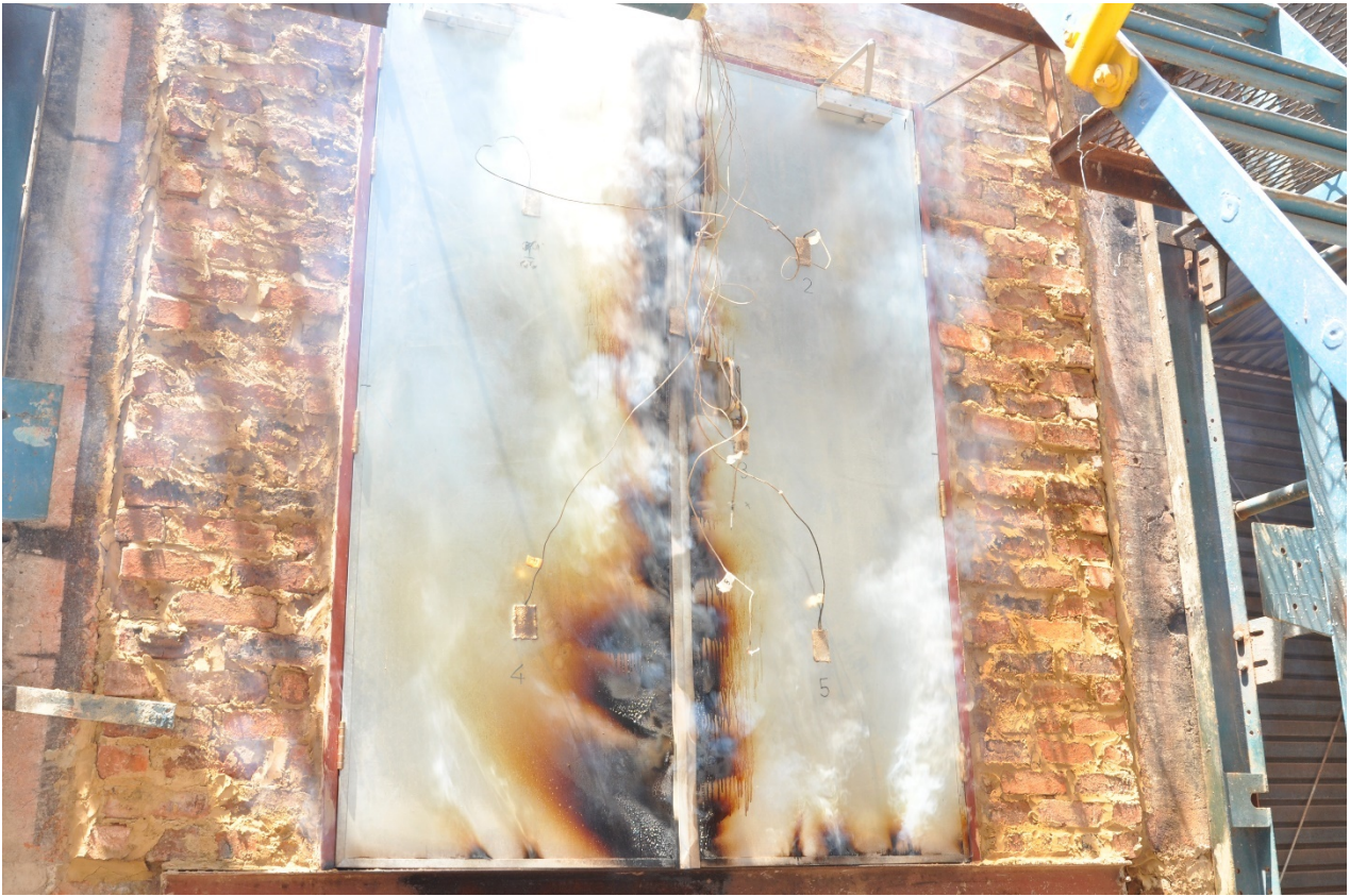
Figure 4.2.5: Discolouration on the door interface
