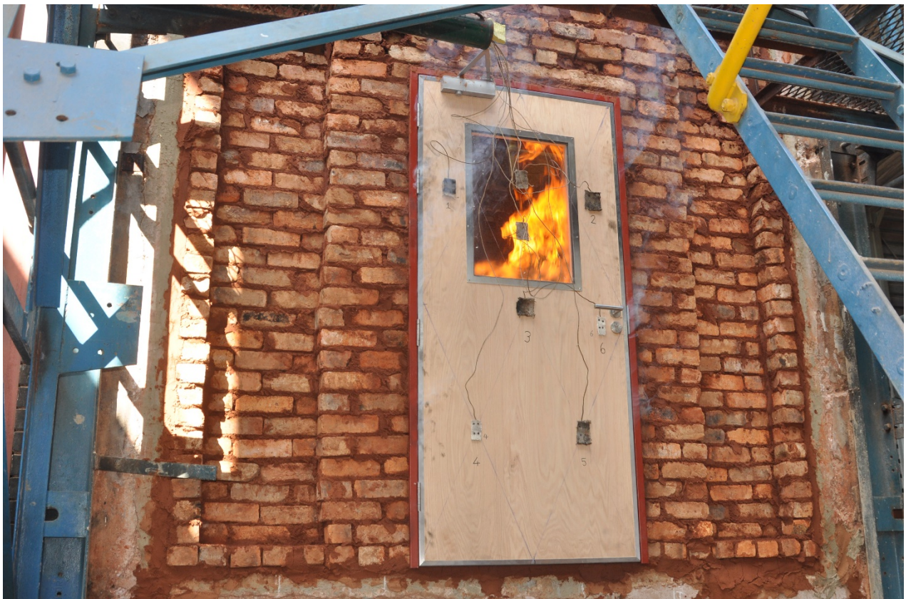
Figure 4.2.4: Door surface aflame inside furnace
