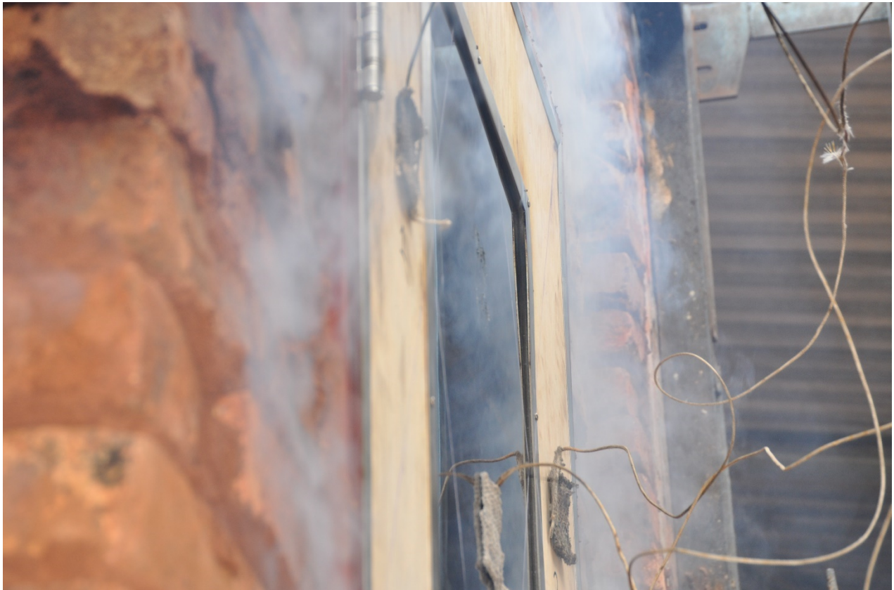
Figure 4.2.11: Material between glass and steel frame expanding
