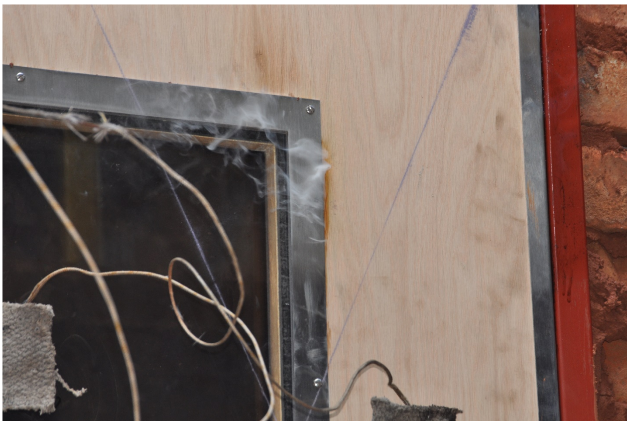
Figure 4.2.8: Discoloration and smoke release on edge of glazing (view panel)
