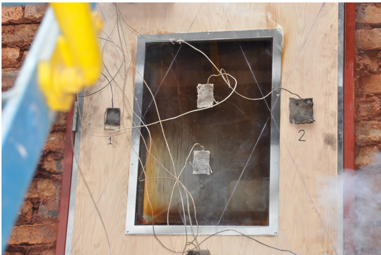
Figure 4.2.9: Condensate forming inside glazing (view panel)
