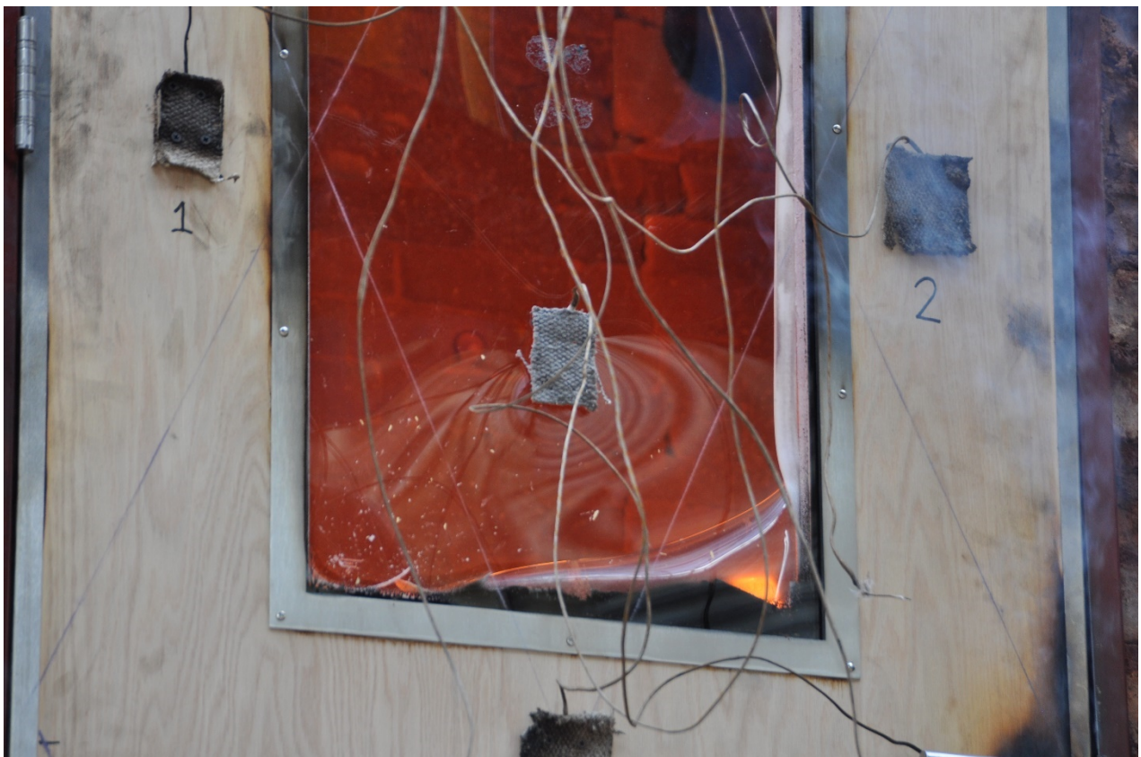
Figure 4.2.14: Glass on unexposed side deforming
