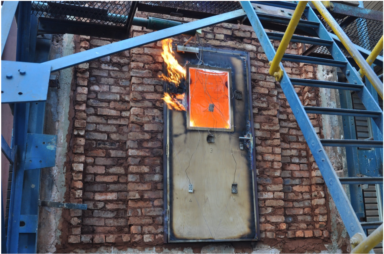
Figure 4.2.19: Flaming rapidly spreading on unexposed side
