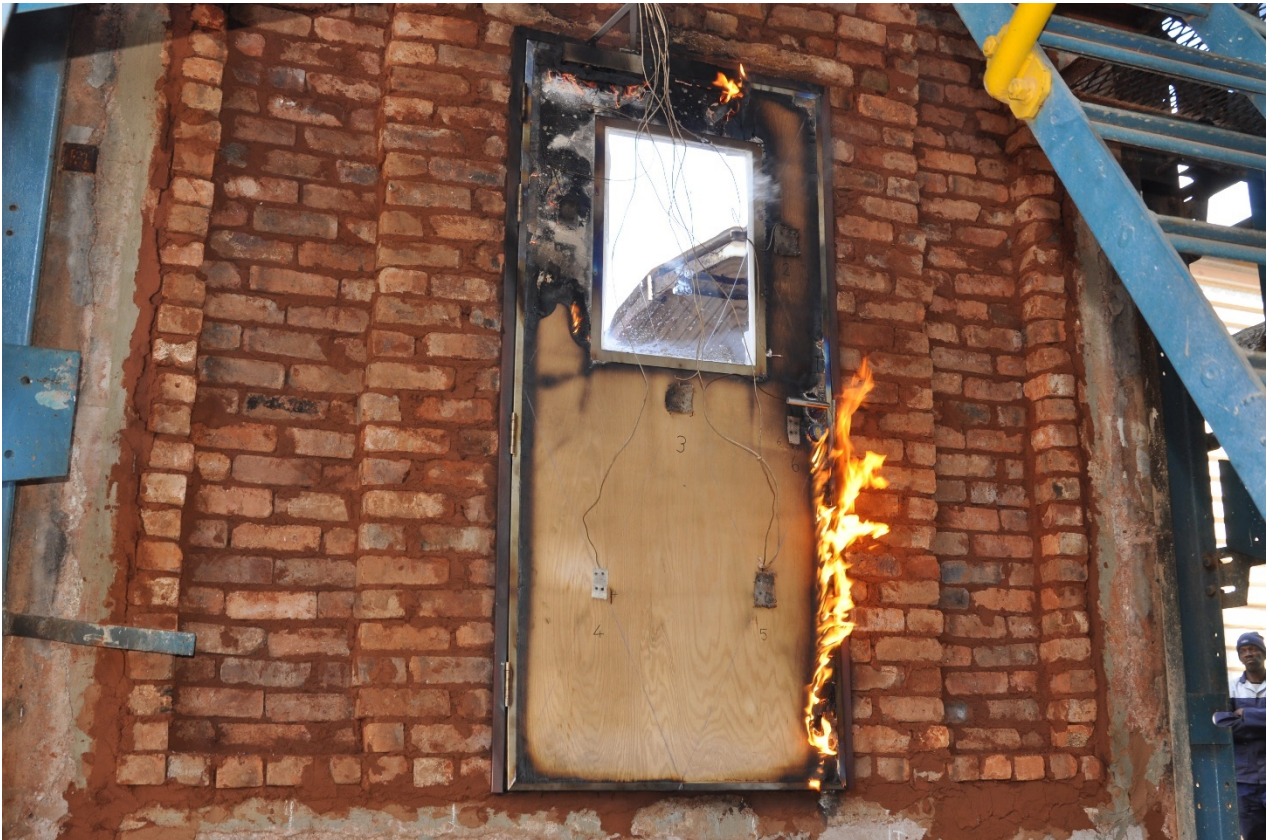
Figure 4.2.21: Unexposed side of specimen at conclusion of the Fire Resistance test
