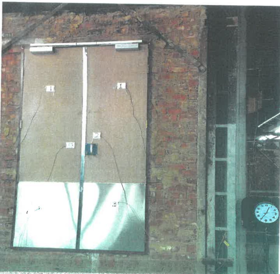
Photo 6: Unexposed side at 35 min, little smoke appearing at the top left corner
